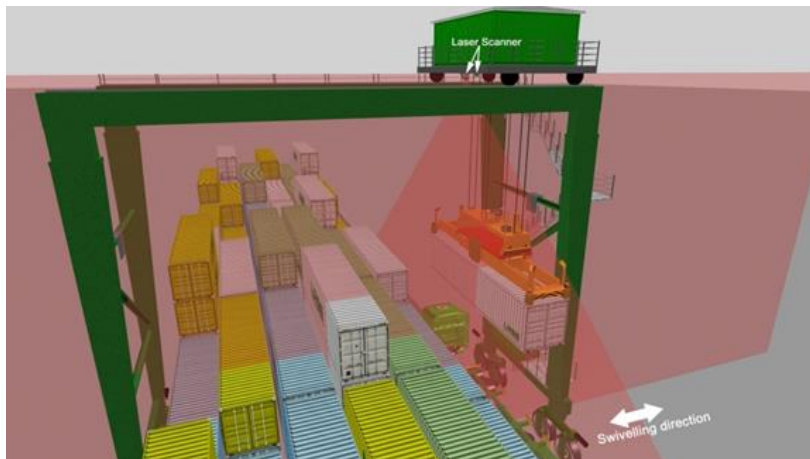
Graphic 4: Crane with scan planes of 2D and 3D laser scanners
