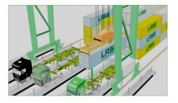
The solution LaseTDS - Twistlock Detection System is built to ensure a fully automated loading and unloading of containers from or to truck-trailers in ASC transfer areas.
