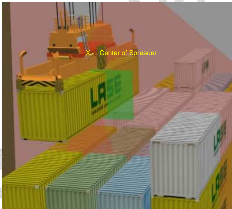
Figure 16: Surveillance field (green) – trolley do not move
