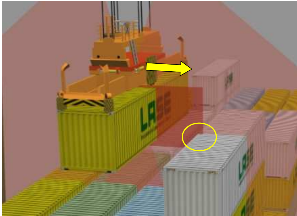
Figure 17: Surveillance Filed – trolley moves to the right (Collision case)
