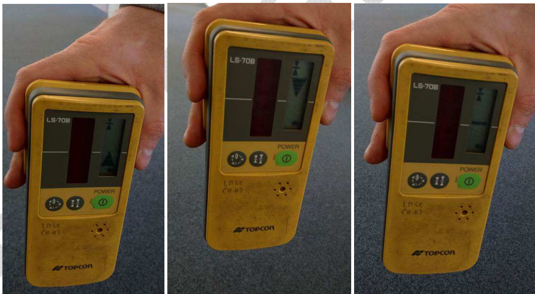
Figure 30: Beam-finder in first figure to low, in second to high, in third the beam is in center (see arrow in display window)
