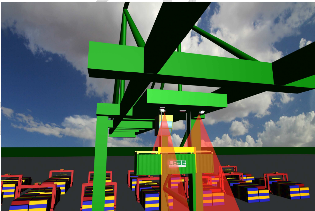
Figure 3: Mounting position of the two laser scanners
