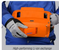
batteries with capacity gauge.
